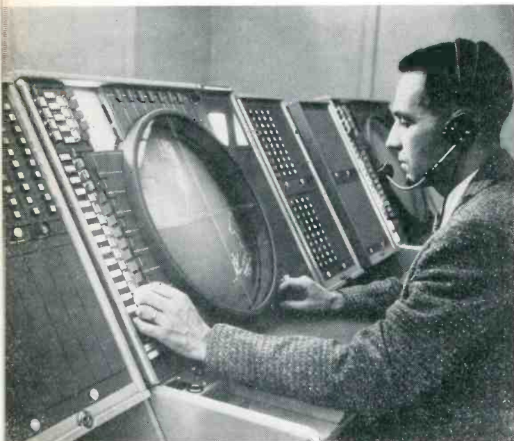
Picture of the air defense situation as picked up by SAGE network and analyzed by IBM computer, is flashed on this screen. With buttons and switches at sides, Air Force personnel make tactical decisions which are in turn carried out by the computer.
