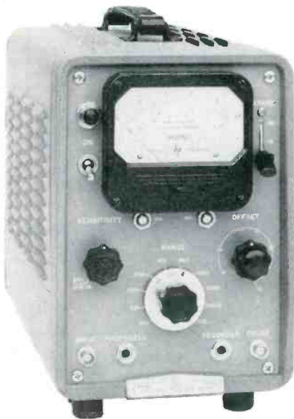
Fig. 1: Discriminator-output frequency meter measures 3 cps to 100 kc
